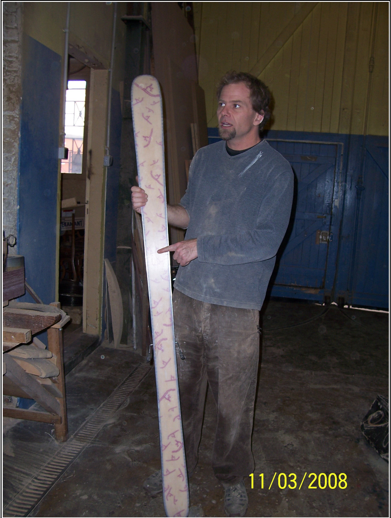
Note the long taper on the forebody and the cool base graphics
